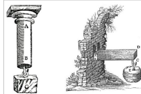
While Galileo is best known for his work on telescopes, astronomy and gravity, he was also very interested in the properties of materials. He devised several thought experiments and practical quantitative tests (see image, right) to better understand the strength and stiffness of different materials. These groundbreaking insights led to the birth of strength-of-materials science, inspiring others like Robert Hooke who further studied elasticity of materials (i.e. *Hooke's law*).
